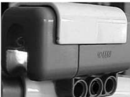
Figure 1: LEDs on a light sensor Either way there are two LEDs (Light Emitting Diodes) on the sensor as shown in figure 1.
