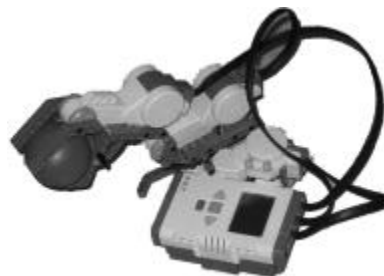
A three motor robot arm using the NXT
