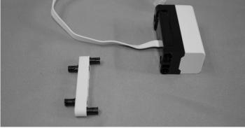
• Insert the 4 short black friction pins into the #7 technic lift arm as shown
