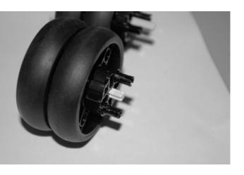
You can increase the strength of the assembly if you replace the two black friction pins with two #3 blue friction pins and have them connect from the inner wheel, through the round block, and into the motor hub.
