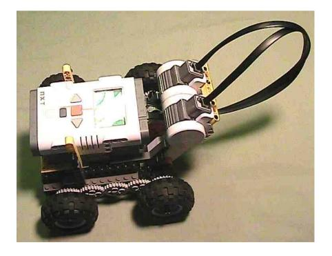
With modification, you can have the motors go straight up, angled back (shown) or straight out the back. Just modify the base used to hold the motors and the NXT together.
