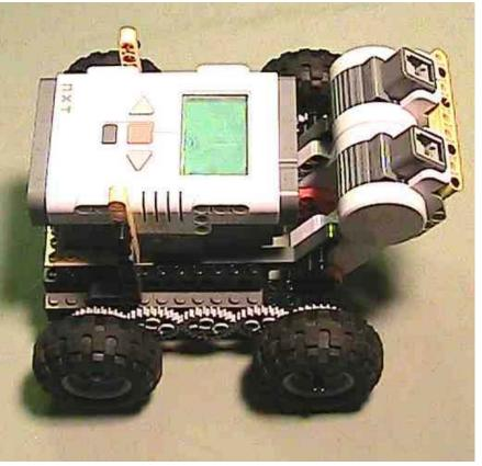
Note: The robot chassis is an even number wide and the NXT is an ODD number of Studs wide, so you have to put a spacer in to "fill the gap" as shown above.
