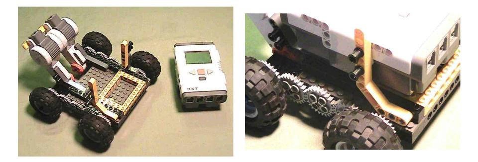
Note: Using long Technic pins with stop bushings allows you to pull the pins out Without taking much apart. Easier on the robot and the fingers.
